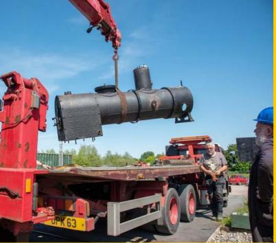
Stage two of the operation was to load up Montalban's boiler for despatch to Johnson's.
