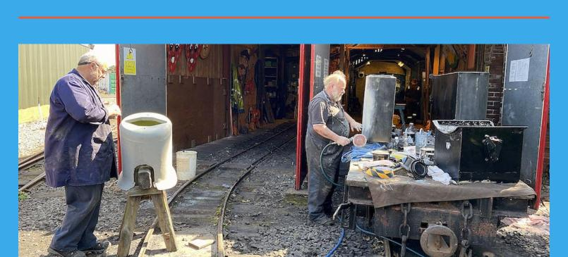
Meanwhile our other O&K locomotive *Montalban* is well on the way towards a return to service. Here the side tanks and the dome are being fettled in the sunshine prior to re-fitting.
