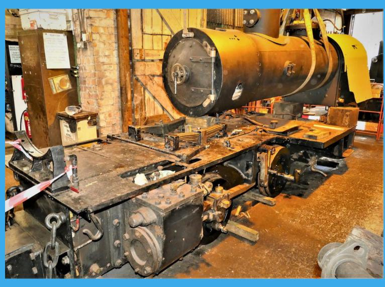
More progress with *Montalban's* refit, with the wheels re-installed and the boiler being lowered back onto the frames.
