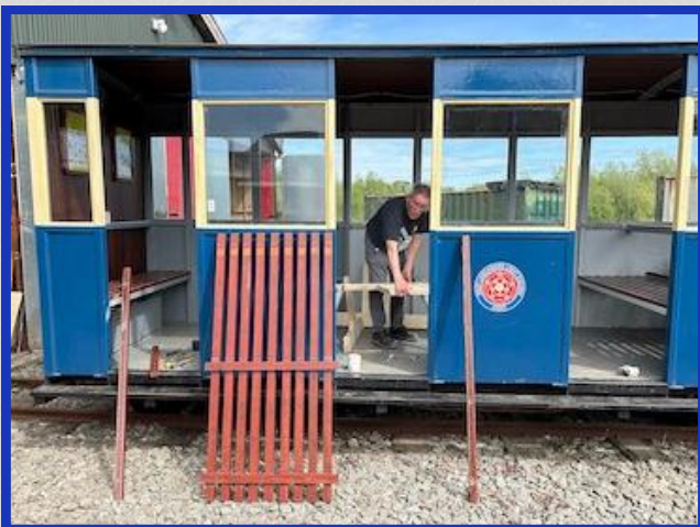
The new coach seats are coming on well, with Jeff putting his joinery skills to good use.
