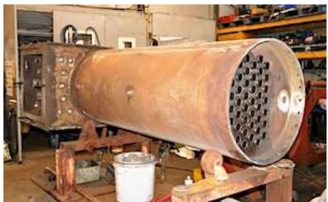
The boiler for our Quarry Bagnall Sybil is nearing completion, with the throatplate/ firebox assembly now riveted to the boiler shell. This work is being done down the road at Johnson's of Banks, who have the facilities we need.
