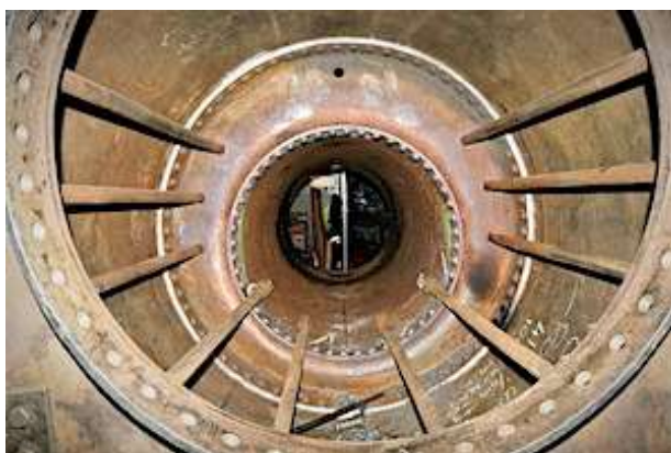
The boiler for our Quarry Bagnall Sybil is nearing completion, with the throatplate/ firebox assembly now riveted to the boiler shell. This work is being done down the road at Johnson's of Banks, who have the facilities we need.
