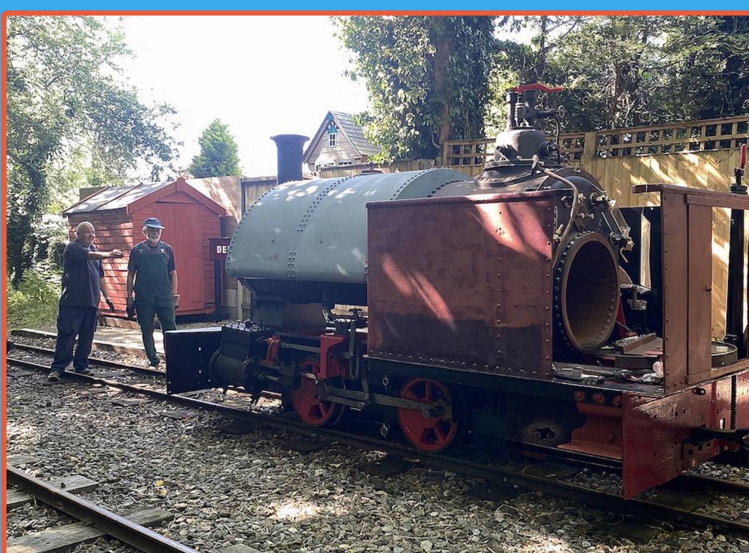
An important milestone in the restoration of our Quarry Bagnall Sybil, as the locomotive is shunted all the way down the line to Delph, to check operation of the motion and various other components. Gordon and Richard cast a critical eye over the proceedings.
