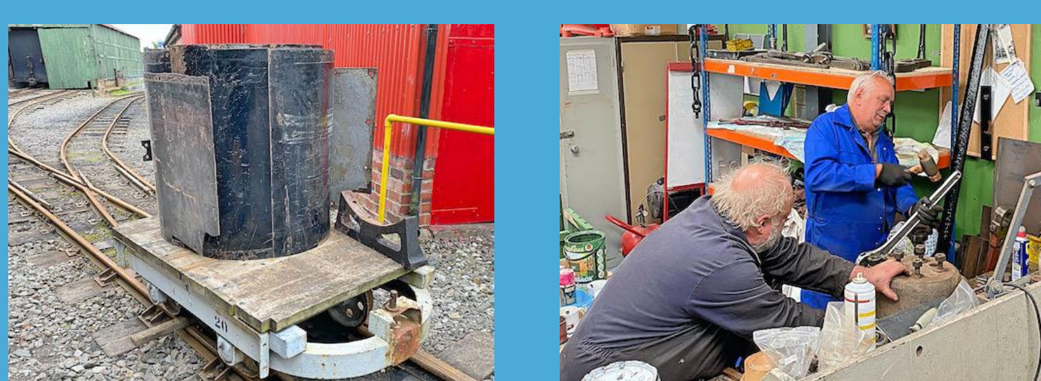
Montalban's boiler wrapper on the move to the shotblaster's, while Keith and Alan wrestle with the steam dome.
