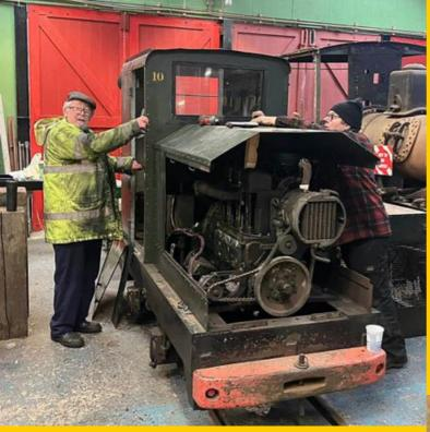
Meanwhile in the mechanical workshops our long-serving diesel shunter *Planet* gets a muchanticipated overhaul. Bob and Dave start by removing the engine covers, overcoming some stubborn resistance from inaccessible and wellrusted bolts.
