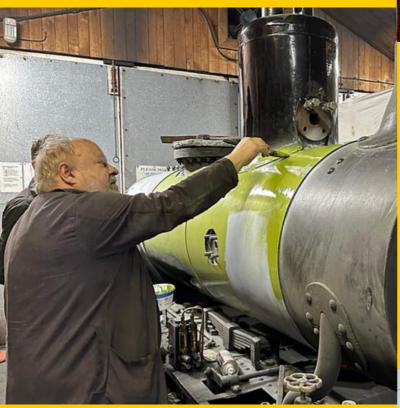
The finishing touches. Simon fettles the regulator valve while Keith does some last-minute brazing on the steam pipe and Cameron tries to keep out of the all-pervading rain.
