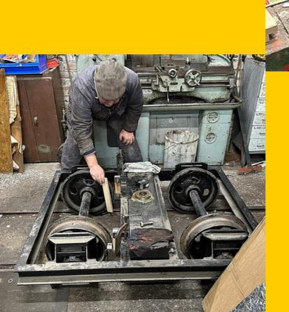
With the topsides of the coach's braking system complete, Paul turns his attention to the components on the bogie. He assures us that the wood is only for dimensioning, the finished articles will definitely be metallic.
